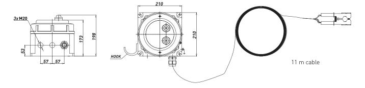
GUMT.. Series - Earthing control system - Copper-free aluminium
